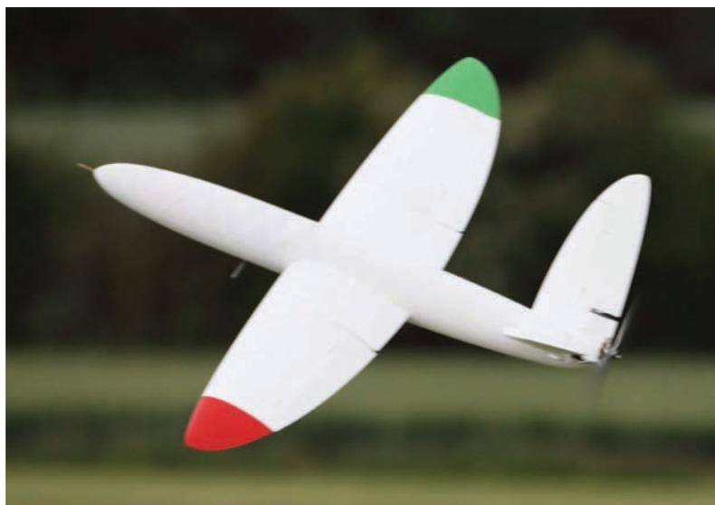
This UAV experiment uses an elliptical wing form, which is traditionally difficult to manufacture but was easily produced through 3D printing
